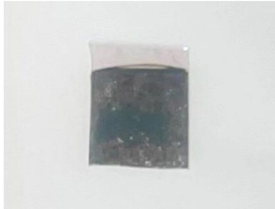
Figure 4: Electrodeposited heterostructured ZnSe/MoS<sub>2</sub>
